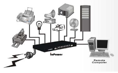
ioPower connected to a host PC
