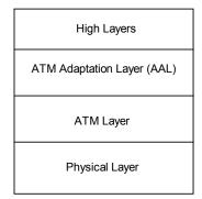
Figure 6: ATM Model Layers
