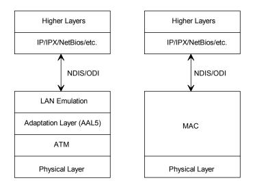
Figure 7: ATM + LANE compared with 802.3 or 802.5 LANs
